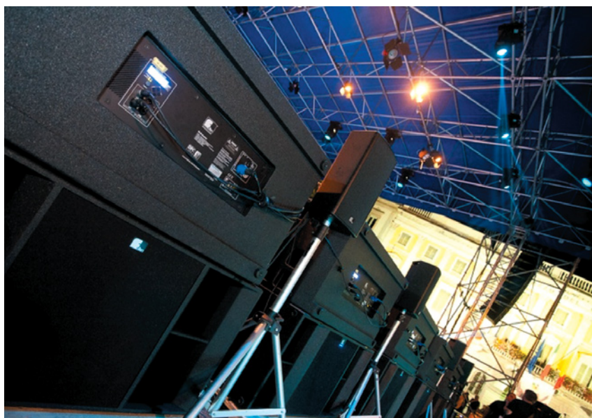
A row of cardioid sub arrays in action, comprised of Fohhn PS9 active subwoofers.
